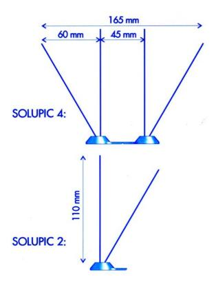
A notch in the middle of the system makes it very easy to change SOLUPIC 4 into SOLUPIC 2.
